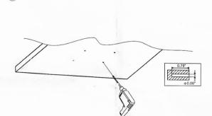
Drill pilot holes where the four marks are located with an impact drill
