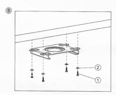
Install the mounting panel with four screws ①and four washers ②.
