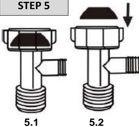
Put the black rubber-washer on top of the 3-Way Valve
