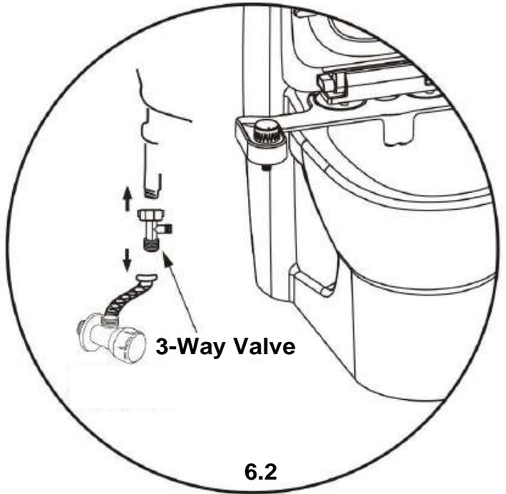
Connect the 3-Way Valve to the toilet water supply as shown in the drawing
