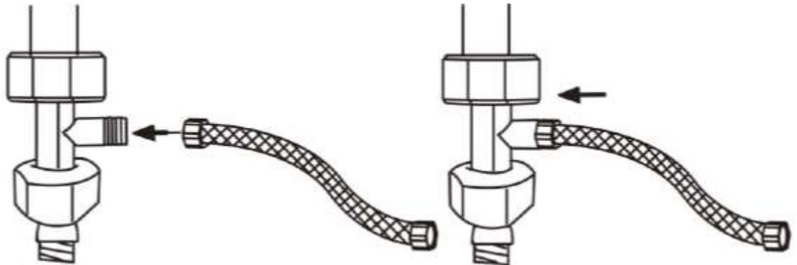
Connect the hose for toilet water supply and the stainless steel braided hose to the 3-Way Valve
