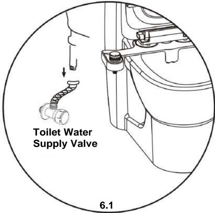
Make sure the toilet water supply valve is closed and the water-tank fully emptied
