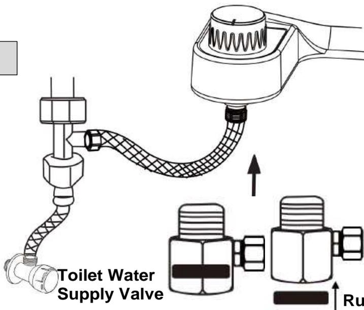
Connect the Stainless Steel Braided Hose to the 3-Way Valve. Make sure not to overwist the thread. Screw the connector on by hand at first and then tighten it carefully for no more than a quarter to half turn with the wrench
