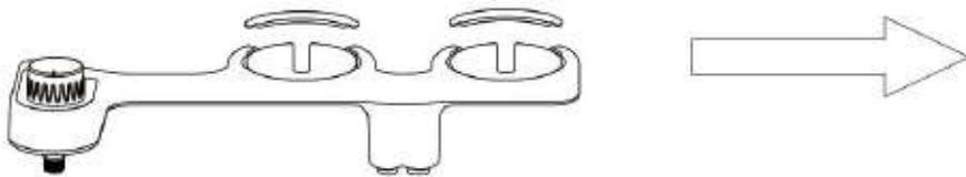
Connect the bidet-extension to the toilet seat and make sure, the pins snap in. Adjust the bidet to make sure the nozzle is positioned in the middle
