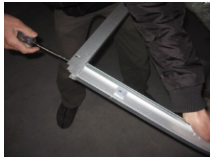
SIDE COLUMN CONNECTED WITH SLIDING PROFILE
