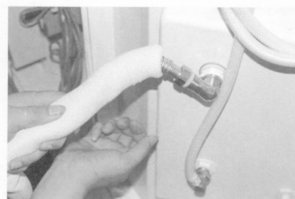
43. Attach the other end of steamer tube on the steam input, tighten it
