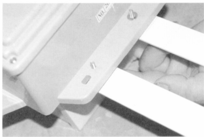
37. Make the steamer generator the same line with steel shelf, fix them by screw
