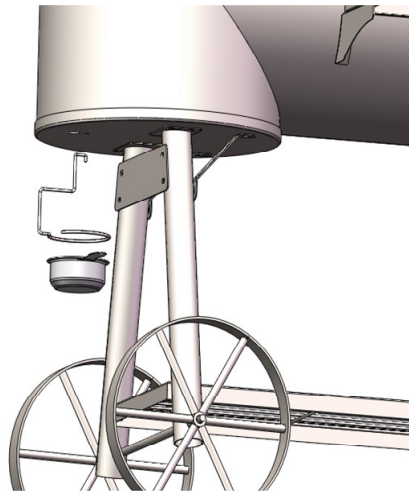
2.24 Assemble the Oil cup and Oil cup hook
