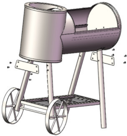
2.7 Assemble the Body Bracket with M6*15 screw and M6 nut
