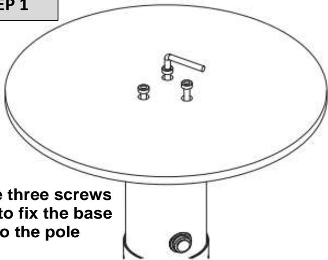
Use the three screws M6x25 to fix the base onto the pole
