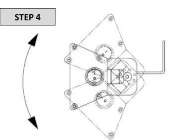
To set the ideal inclination angle, please loosen the two M6x10 Screws, position the heater as requested, and retighten the screws
