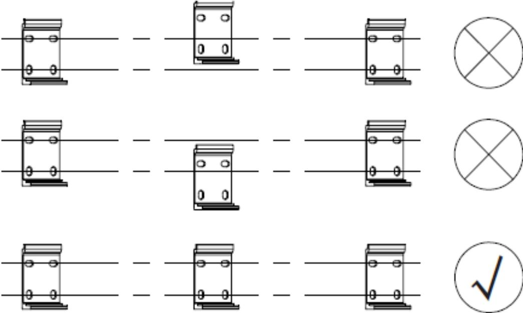
To avoid problems due to incorrect positioning, please make sure to use the **Adhesive fitting templates** as described on page 11, step 2 (Positioning the wall brackets)
