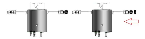
\*Note: The length of AC cable on microinverter is roughly 2 m, if the distance between two microinverters is more than 2m, please use an AC extension cable between two microinverters (as shown in the picture below).
