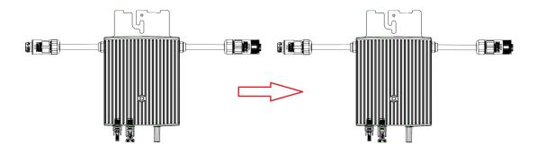
B). Install the AC end cap on the open AC connector.
