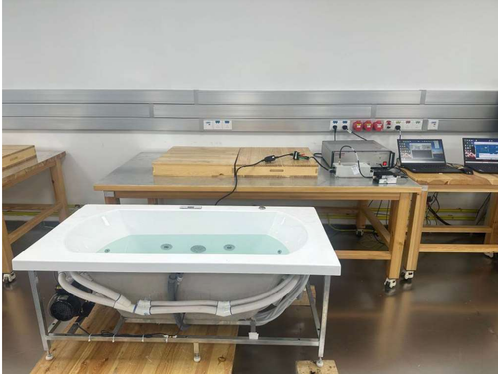
Photograph 7: Set-up for Injected Current
