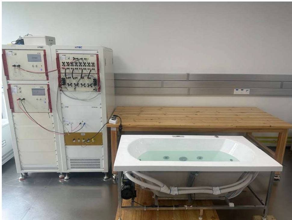
Photograph 5: Set-up for Surge
