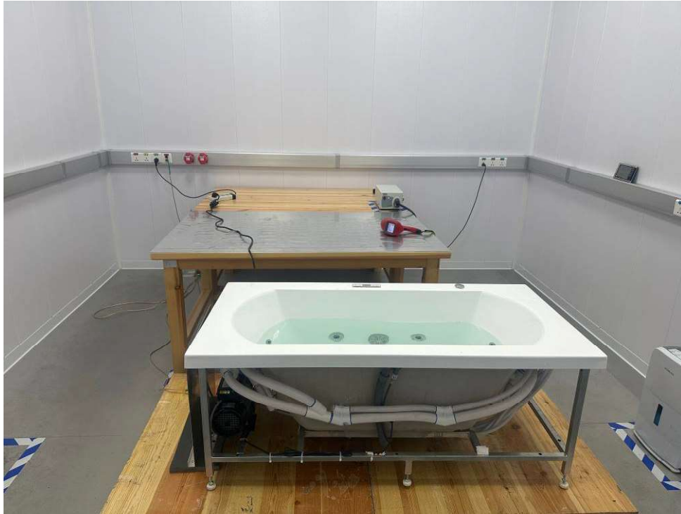
Photograph 4: Set-up for EFT
