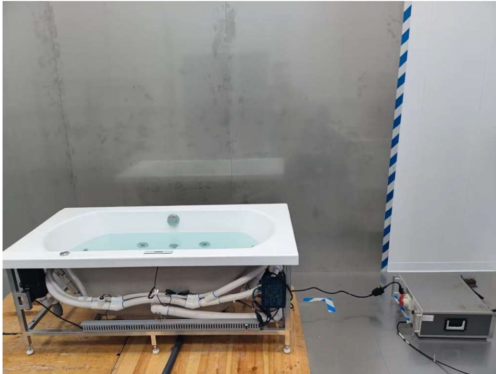
Photograph 1: Set-up for Disturbance Voltage
