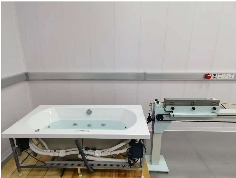
Photograph 2: Set-up for Disturbance Power
