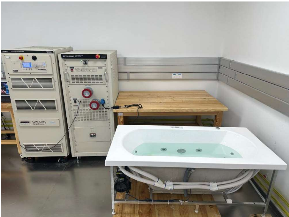
Photograph 8: Set-up for Harmonic and Voltage Fluctuation and Flicker
