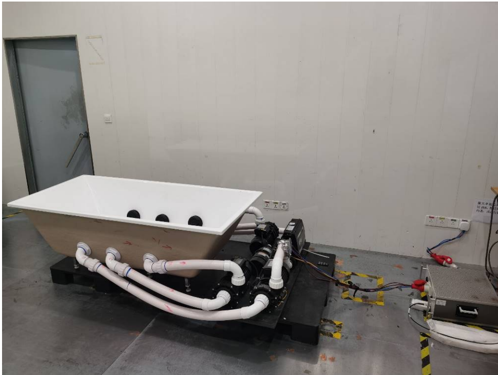
Photograph 1: Set-up for Disturbance Voltage
