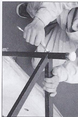
9. Use the adjustable spanner to tight all the pillars with M10x40mm screw.
