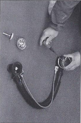
52. Loosen the switch handle with screwdriver as pic shown.
