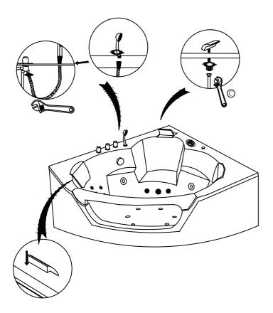
3. Move the bathtub to the wall corner; put the drainer into sewer and seal the drainer. Adjust the tub feet to make the bathtub horizontal. Seal the gap between the bathtub and the wall with sealant to avoid water leakage.
