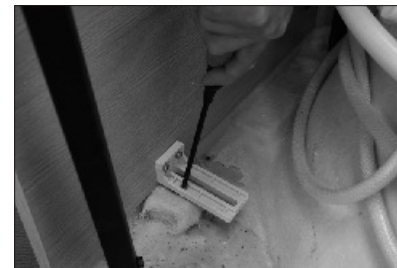
11. Tighten the screw to make sure the "L" shaped connector connects well.
