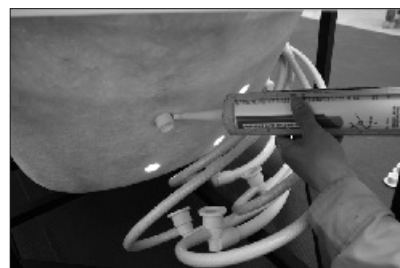
11. Insert the small water jet to the tub and seal with silica gel around it from back side.
