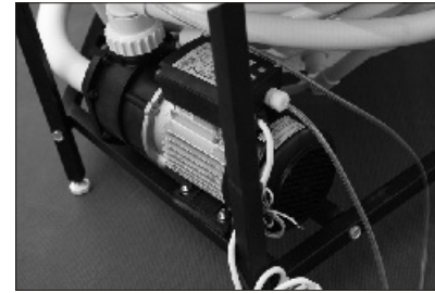
67. Insert one end of air pipe to the control box as pic shown.
