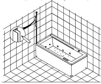
3.Make the hole as prepared by electric drill in the wall, knock the expansion plastic material into the holes
