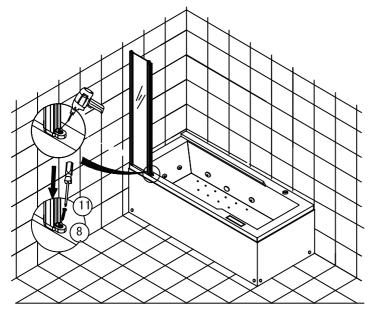
6.Connect the active glass and fixed glass with glass door connector, and fix it with 4\*40 self-tapping screw.
