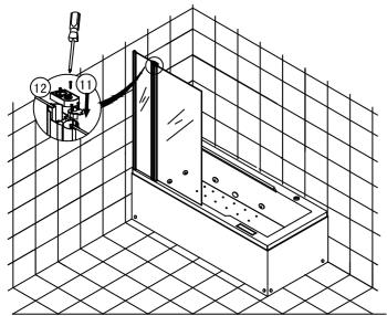
7.Adjust the depth of glass door wedging in the aluminum profile., make the glass door gap accordance. Drill a hole on the aluminum alloy profile in the diameter of 3.2. Fix the glass door by 4\*12 self drilling tapping screws with cap.. then install the waterproof tape
