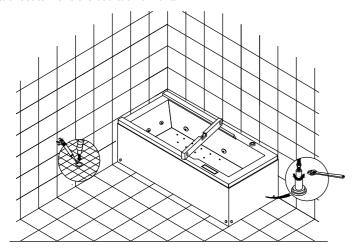
2. Put the profile against the wall onto the bathtub(ten Millimeter distance from the wall), mark the position of drilling hole with mark pen.
