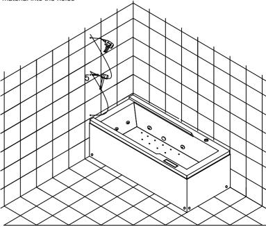
4.Fix the aluminum alloy profile on the wall with 4\*40 self - tapping screws.
