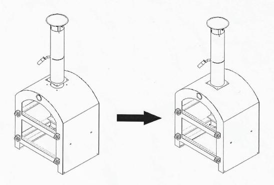
Step7: Connect handle to oven body by 2 pieces M5\*10 screws and 2 pieces  $\phi$  6 spacers 、 2 pieces silicon rubber spacers. The silicon rubber spacers should be between the handle and body.
