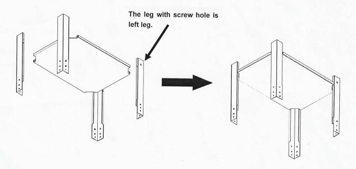
Step 2: Connect the Step1 part to Trolley's top plate by 16 pieces M5\*10 screws
