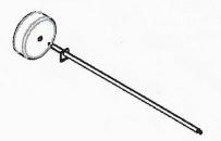
Step4: Connect step2, step3 part to another wheel by one  $\Phi$  6 spacer and 1 piece M6 screw nut
