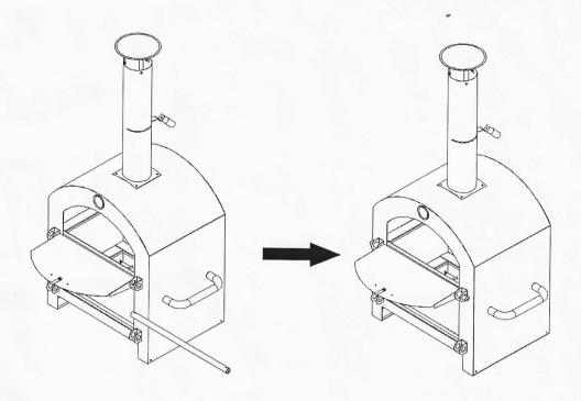
Step9: Connect under door to Step 8 part by 2 pieces R plug and 1 piece door spindle
