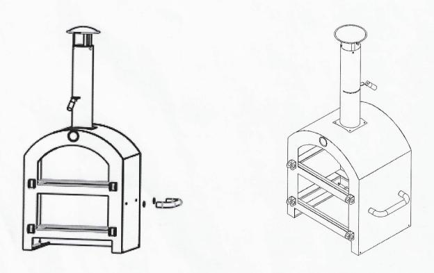
Step8: Connect up door to Step 7 part by 2 pieces R plug and 1 piece door spindle
