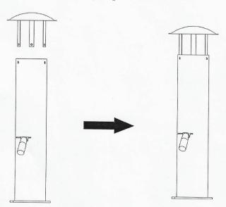
Step6: Connect Step 5 part to oven body by 4 pieces M5\*10 Screws.
